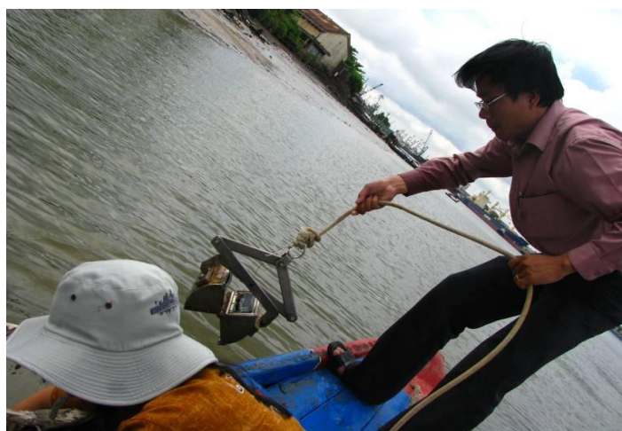
Fig. 3.3 Sediment sampling by Petersen grab.
