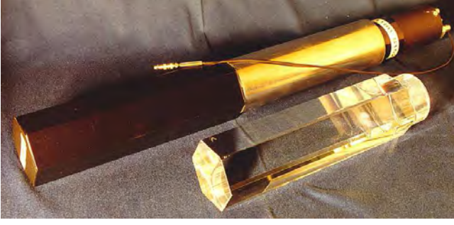
Figure 3.16: Single BaF 2 module of the TAPS spectrometer and a scintillator crystal.
