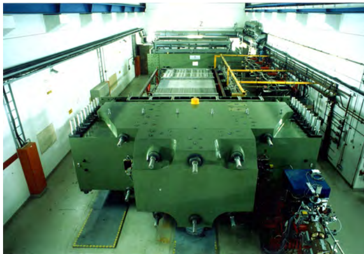
Figure 3.3: The 3rd race-track microtron (RTM3) of MAMI-B. Each of the two bending magnets weighs 450 t.
