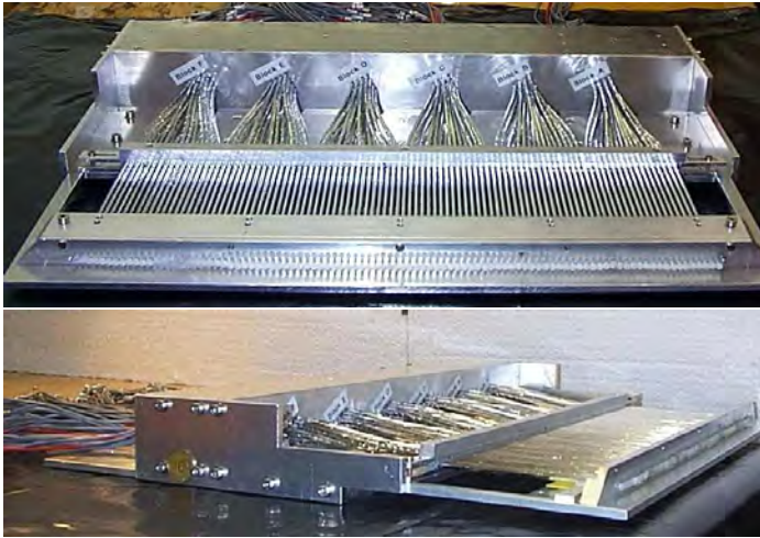
Figure 3.5: Finished tagger microscope detector assembly without black plastic wrapping.
