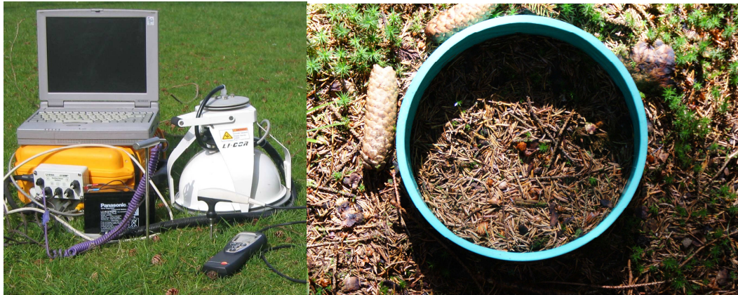
Figure 12: LICOR-8100 measurement chamber (left) and plastic collar for soil respiration (right) (own photo material)
