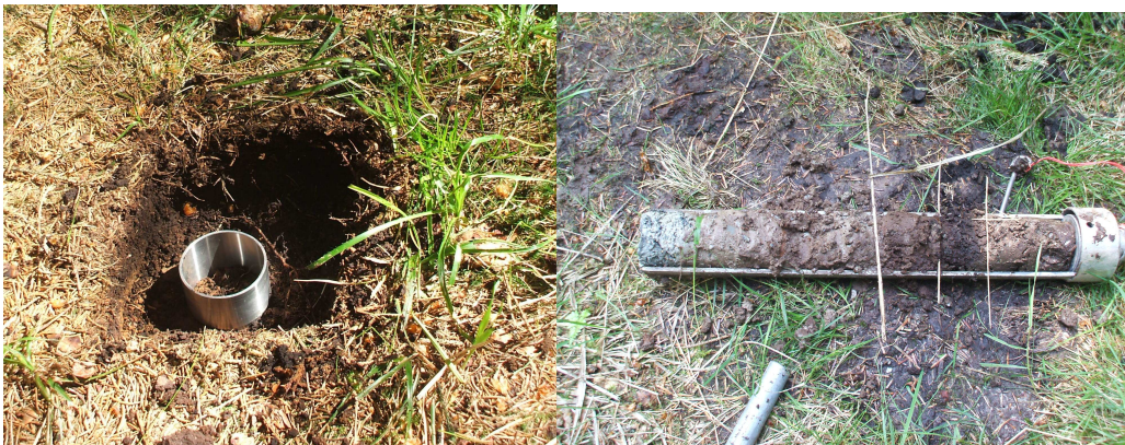
Figure 14: Metal cylinder used for bulk density analysis (left) and soil core (right) (own photo material)
