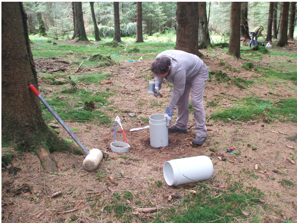
Figure 10: Installation of collars used for root exclusion (photo by Guido Sciuto)
