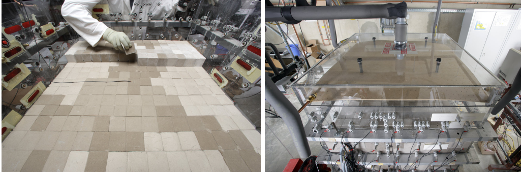
Figure B.4: Left: frozen cubes are packed into the sandbox; right: view at the evaporation chamber.
