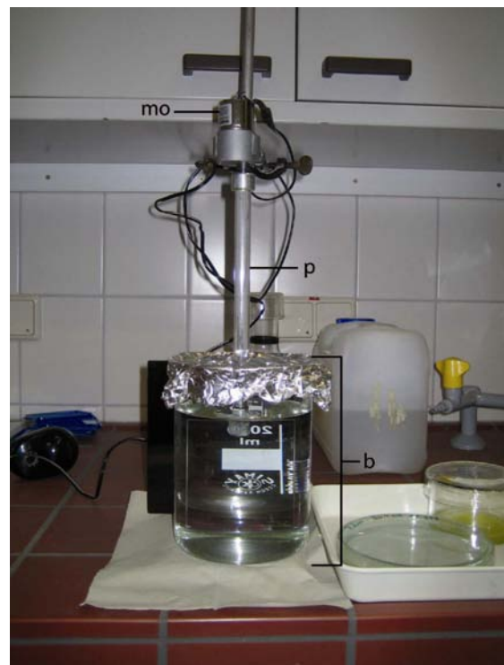
Figure 4: Installation of equipment in the cooled laboratory at the Freie Universität Berlin for cultivation of larvae. b beaker, mo motor, p shaft of paddle.
