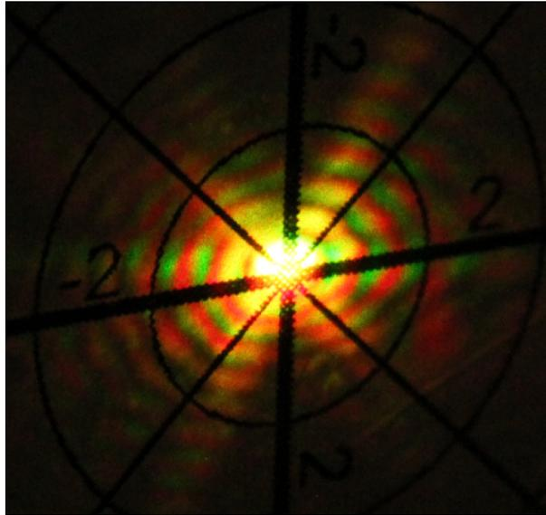
**Figure 4.4:** Diffraction of a red and green laser beam at a pin hole projected onto a screen.
