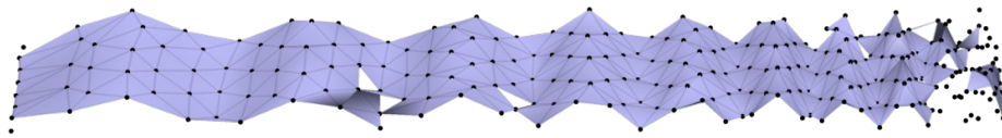
Figure 7.7: Triangulation of the sparsely sampled surface from Fig. 7.6a with the algorithm from Amenta et al. (2000). Especially on the right-hand side the sampling density is too low for a correct triangulation.
