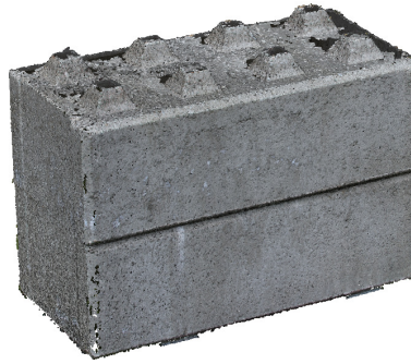
(b) Reconstructed point cloud
