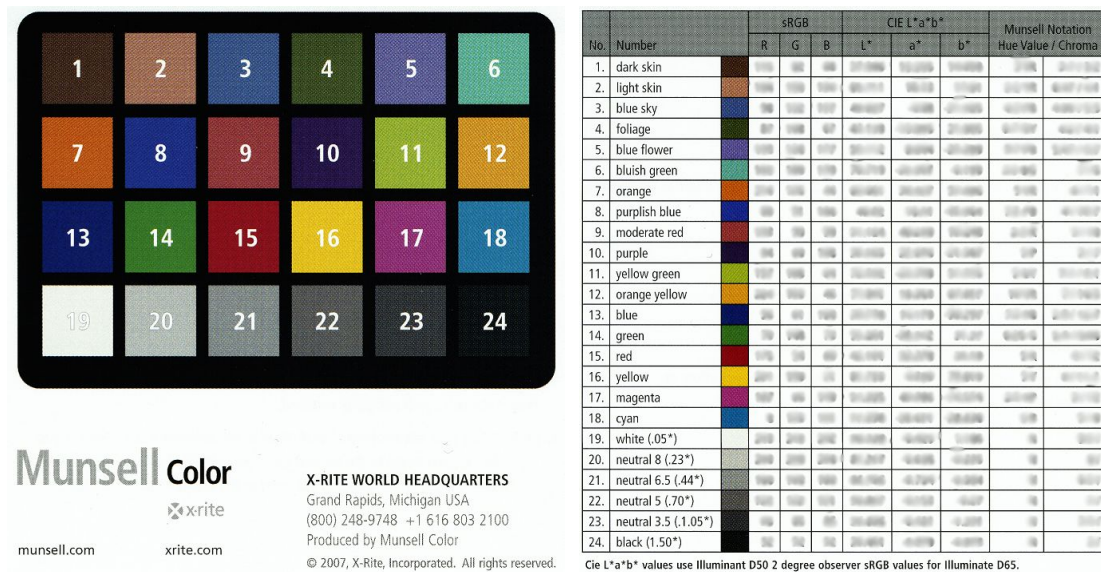
Figure 2.12: Left: Reference X-RITE color checker; Right: table of the corresponding color values as both sRGB and CIE L*a*b* triplets, located on its backside. Note: numerical values were blurred out because of copyright reasons
