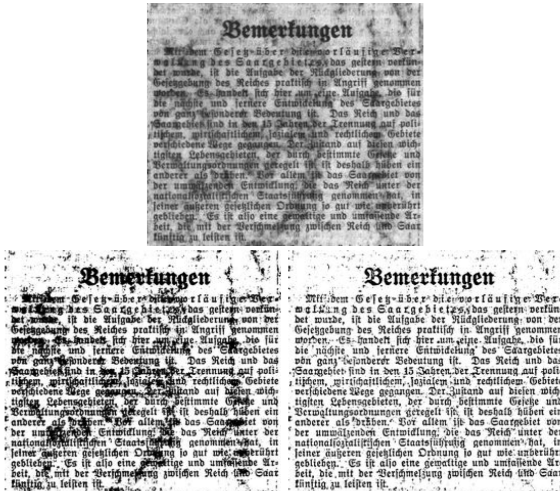
Figure 3.4: Top: Section of a grayscale document image showing significant degradation effects; Bottom: results of applying two different binarization algorithms – Otsu’s optimal global method [204] (left) and the Sauvola et al. [230] adaptive method (right)
