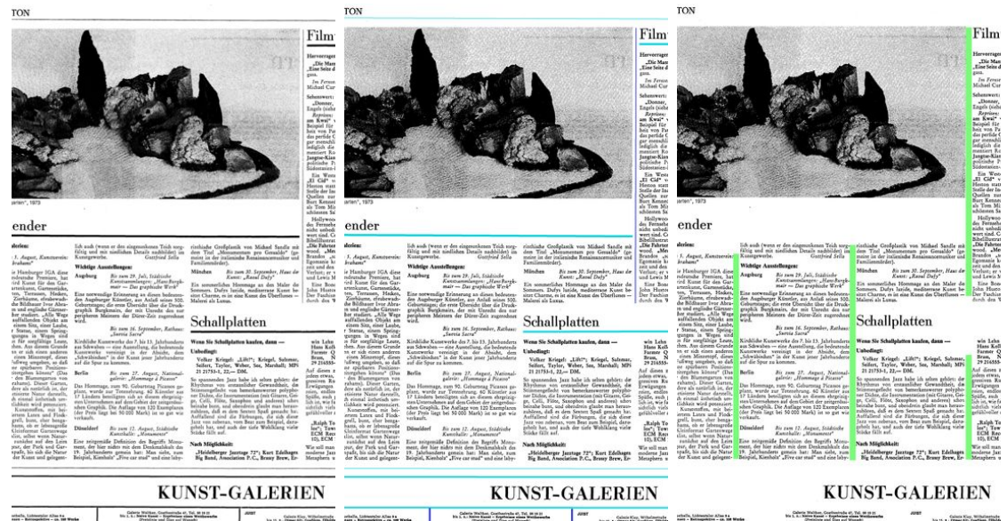
Figure 5.2: Examples of separator types found in documents: left – original portion of newspaper scan; center – solid separators (cyan= horizontal; blue= vertical); right – vertical whitespaces (green)
