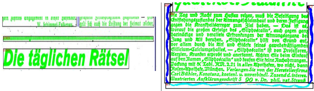
Figure 5.13: Results of solid separator detection: left – missed dashed horizontal separator (labeled as text due to the regularity and size of the dashes); right – correctly labeled wavy separators (green: text, cyan: horizontal separator, blue: vertical separator)
