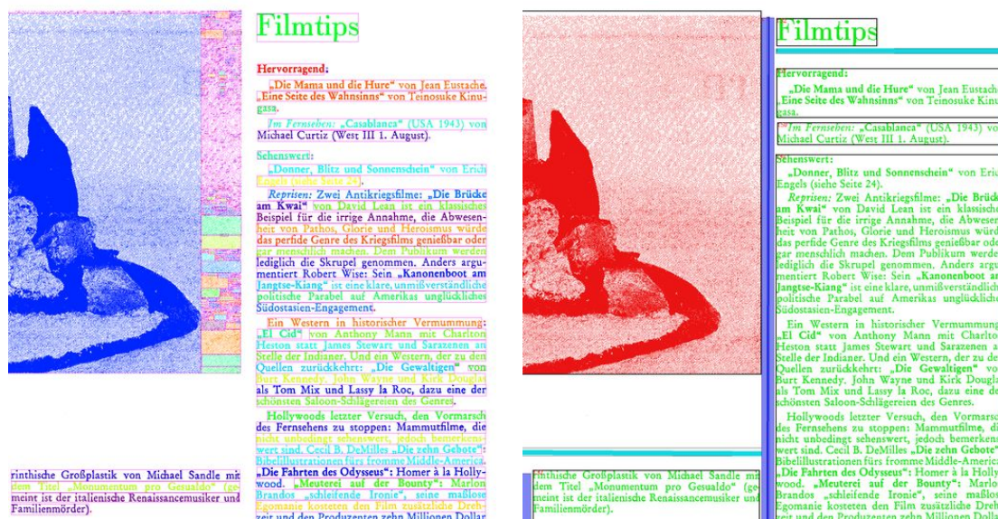
Figure 5.10: Left: GTLs created from the connected components of a document image; Right: region blocks created from the GTLs (green: text; red: non-text; blue: vertical separator; cyan: horizontal separator)
