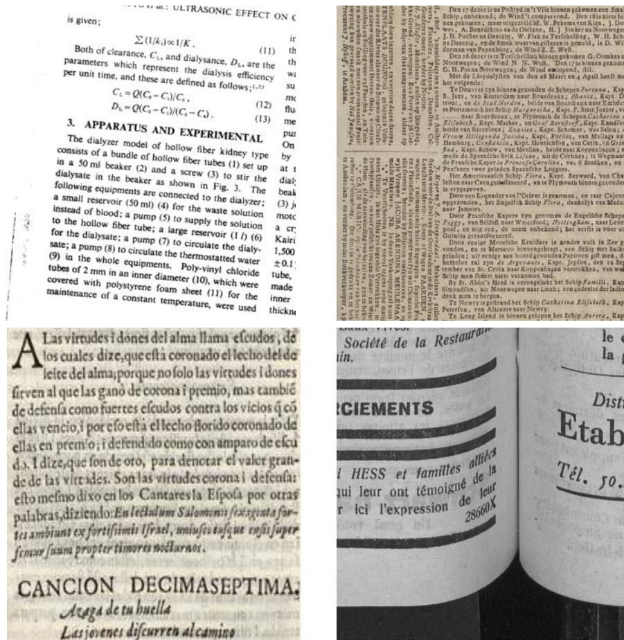
Figure 4.1: Different types of skew found in document scans: global skew (top left), multiple skew (top right) and two common instances showing non-uniform skew (bottom)
