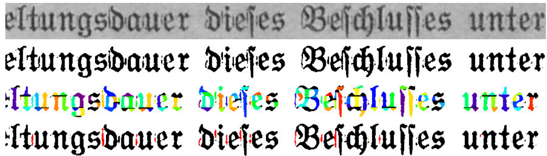
Figure 2.20: Illustration of the proposed character enhancement algorithm's steps. Top to bottom: original grayscale text line; result of binarization using Otsu's method [204]; superimposed initial vertical DSCCs; determined true artifacts (red)
