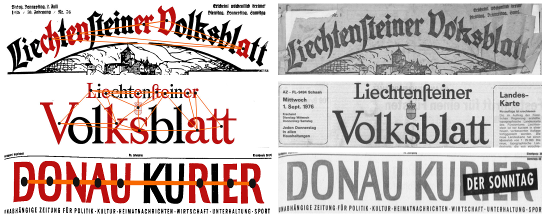
Figure 6.7: Three front page graph models (left), each along with a correctly recognized candidate, illustrating (top-to-bottom): resilience to limited distortions, scaling, partial occlusion
