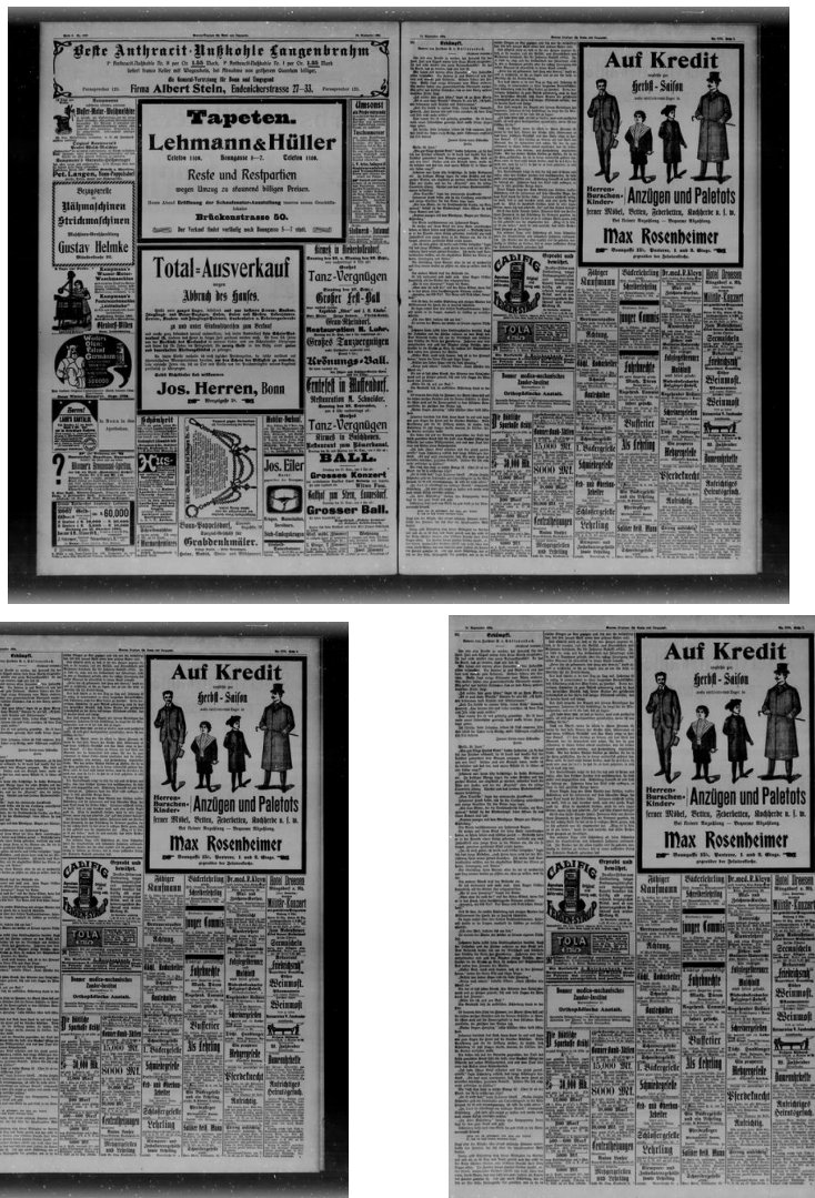
Figure 1.6: Top: Original scan showing two adjacent newspaper pages; Bottom-left: automatic page splitting result for the right-side page; Bottom-right: Border removal and book fold-based deskewing result on the same newspaper page
