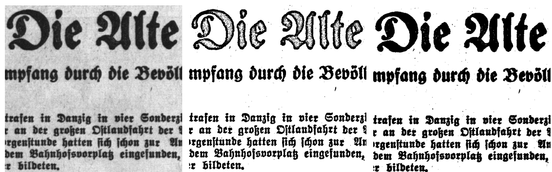
Figure 3.5: A 585 \times 561 grayscale image (left side) and results produced by the algorithm of Sauvola et al. with a window diameter of 19 pixels (center) and 85 pixels (right side). Note the hollowed out large characters produced when using a small window radius in comparison to the character size
