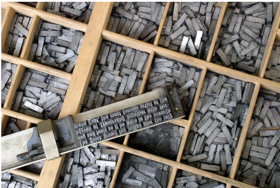
Figure 2.17: Composing stick with a partially finished type directly above a type case. Source: Willi Heidelberg
