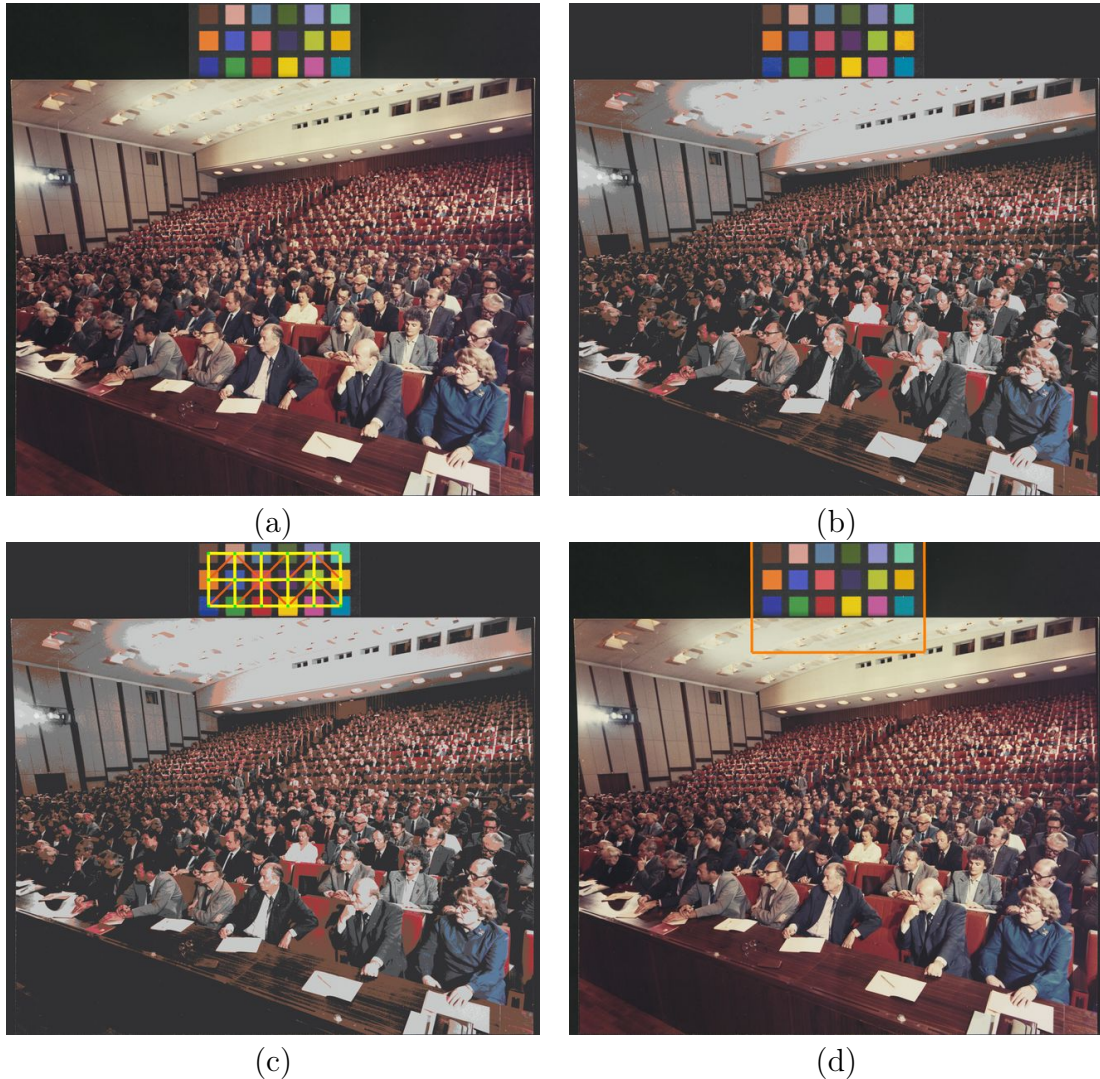
Figure 2.8: (a) Original photograph scan with a completely occluded last color checker line (no grayscale patches visible); (b) after color quantization; (c) with superimposed Delaunay triangulation (orange-painted edges were discarded from the adjacency list used for matching); (d) correctly detected color target
