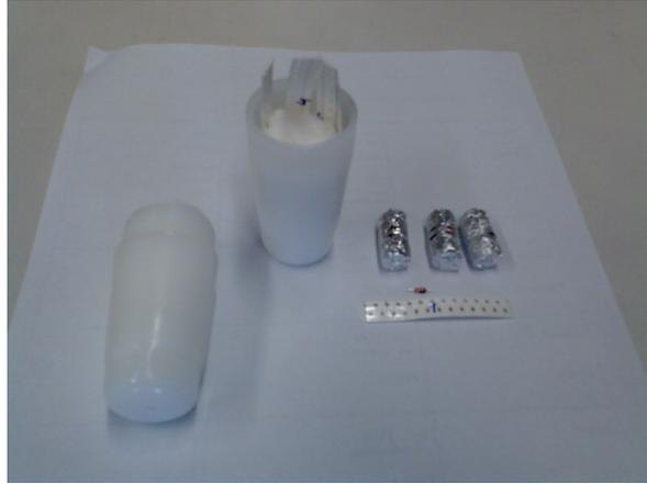
**Figure C.1.:** Photograph of the irradiation sample cartouche. The cartouche itself consists of polyethylene to withstand the high neutron flux in the reactor core during irradiation. It is injected into the core pneumatically via a pipe system and remains at a defined position until the end of the dose application.
