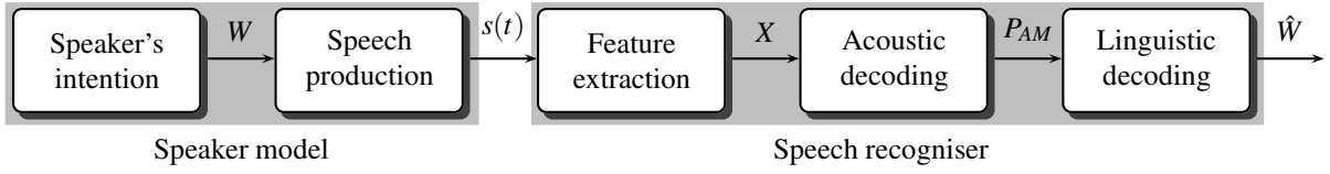
Figure 2.6: Diagram of statistical ASR work flow (adapted from [35]). A speaker has the intention to utter a word sequence W producing an acoustic speech signal s(t) . This signal s(t) is captured and speech features X are extracted. Acoustic decoding determines the acoustic probabilities P_{AM} , linguistic decoding incorporates additional linguistic probabilities and the maximum-likelihood hypothesis for the word sequence \hat{W} is estimated.
