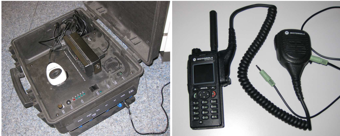
Figure 3.1: Motorola CM 5000 radio station (left) and Motorola MTP 850 hand-held device (right). The TETRA equipment used to record actually transmitted speech is shown in these photographs. Clean speech from the AM Corpus is fed to the line input of the hand-held device, transmitted to the TETRA station, and recorded from the line output.
