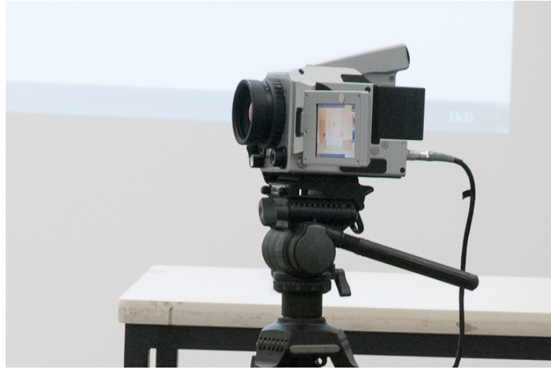
Figure 3.20: Thermal camera VarioCAM © hr Research used for data acquisition.
