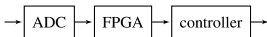
Figure 4.1: Processing chain of an FFTS board. The arrows indicate the data flow. Control is performed the opposite direction.
