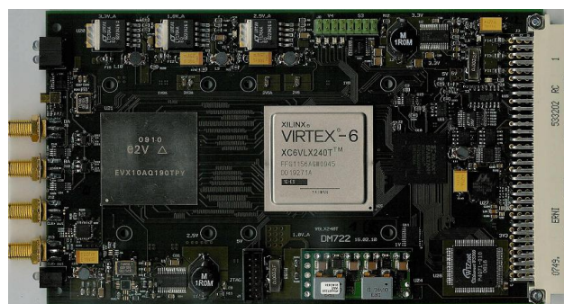
Figure 4.3: Custom-built X FFTS board with a 5 \text{ GS s}^{-1} ADC, a Virtex-6 LX-240T FPGA for FFT and a Spartan-3 1000 FPGA for controlling.
