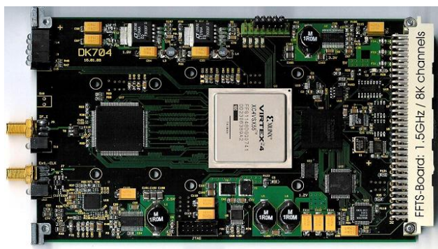
Figure 4.2: Custom-built A FFTS board with a 3 \text{ GS s}^{-1} ADC, a Virtex-4 SX-55 FPGA for FFT and a Spartan-3 1000 FPGA for controlling.
