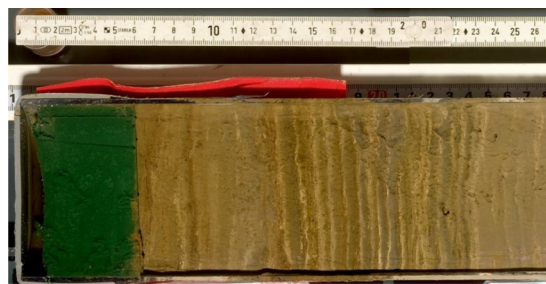
Fig. 4.1: Lake Kinneret; core segment Ki10_V1_top, uppermost 25 cm laminated sediments; scale unit [cm]
