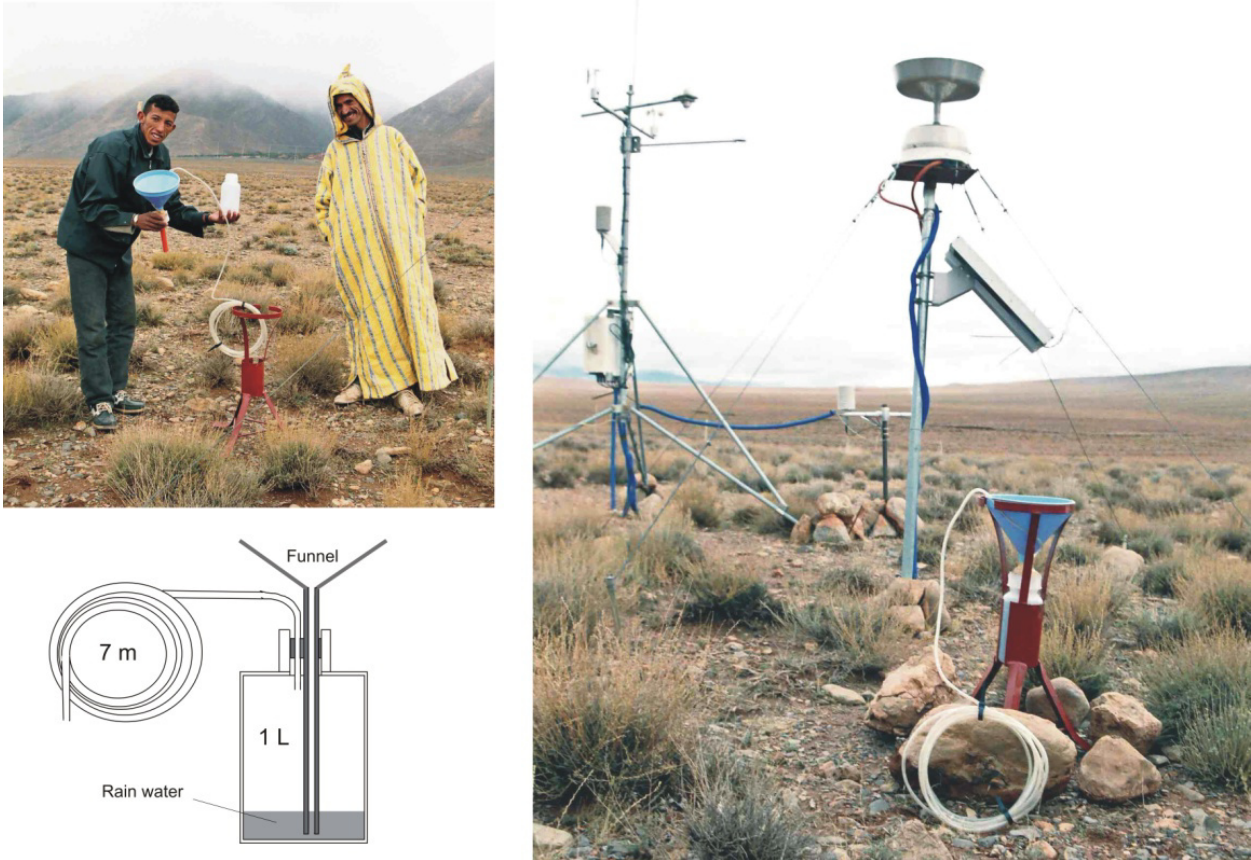
Figure 5-3: Scheme and illustration of a funnel collector to sample precipitation for stable water isotope analysis (from Cappy, 2006).
