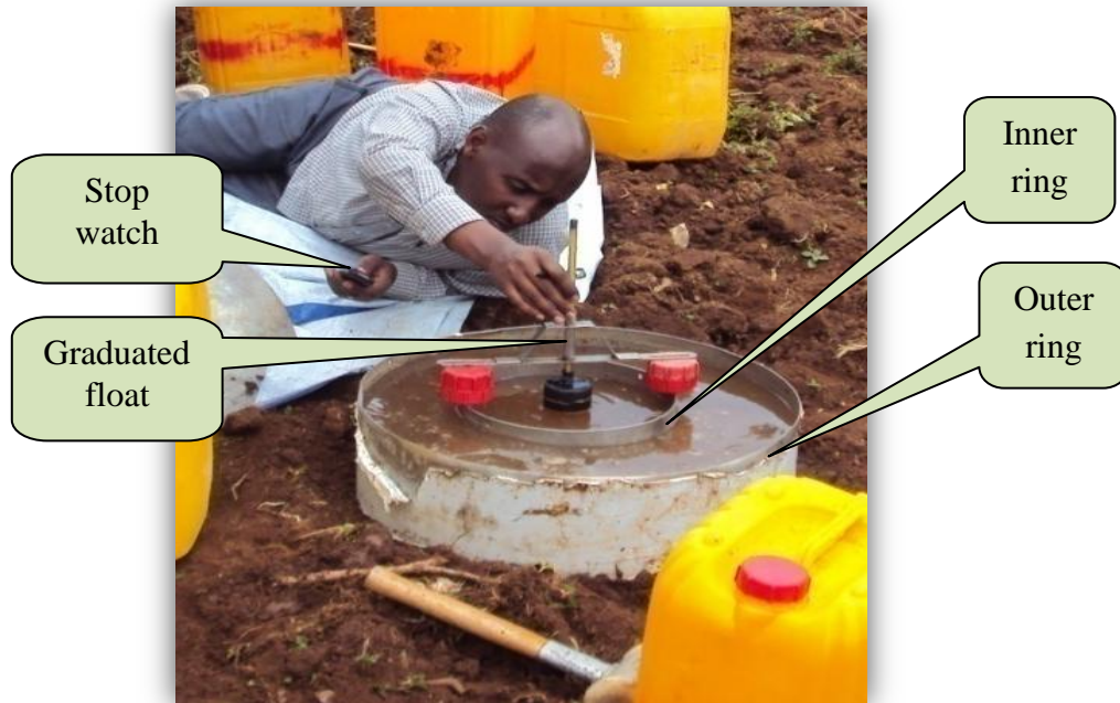
Figure 7.1. Field measurement of infiltration capacity using double-ring infiltrometer
