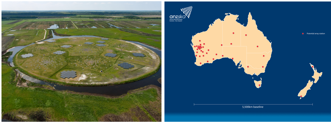
Fig. 6.5: Left: LOFAR 'superterp' in the Netherlands on which six LOFAR stations are housed (image credit: Top-Foto, Assen). Right: Potential SKA array station placement in Australia and New Zealand indicating the 5,500 km baseline (image credit: CSIRO).
