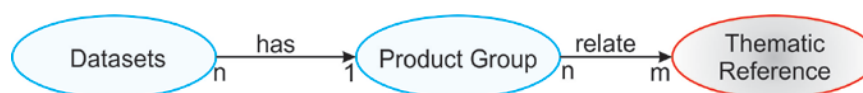
Figure 4.6: The relationship between dataset and thematic reference via product group (Source:(Klinger et al. 2010))
