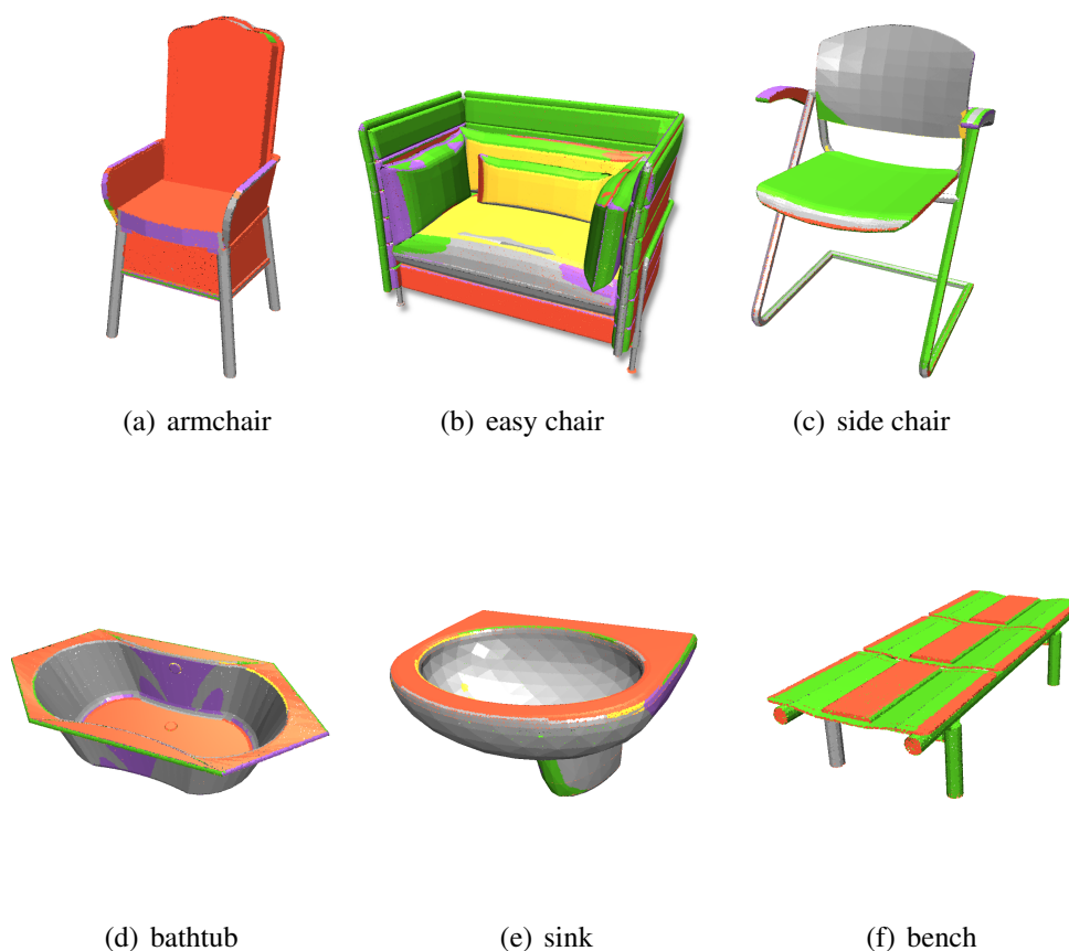
Figure 3.1: Detection of primitive shapes. Colors are chosen with respect to the partially detected primitive types including plane (red), cylinder (green), torus (grey), cone (purple), and sphere (yellow). Figure f) shows an example for the instability of the shape detection. Two legs are identified as a cylinder, but one is identified as part of a torus.
