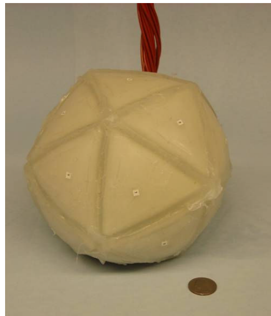
Figure 4.1.: Jamming skin enabled locomotion (JSEL) topology both unactuated (left) and actuated with a subset of the cells jammed (right). Figure taken from Steltz et al. [91].
