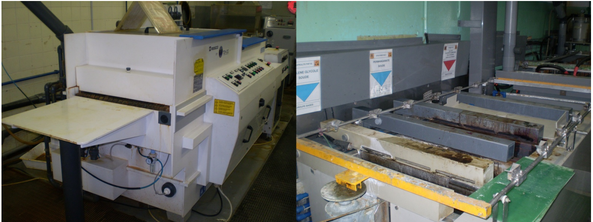
Figure 2.6: Copper-etching machine and baths for chromium removal.
