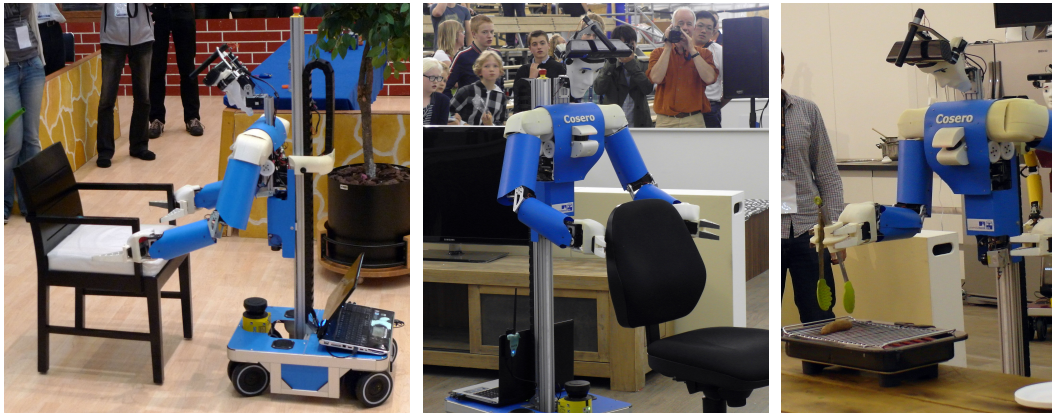
Figure 6.18.: Public demonstrations of object tracking for visual servoing in mobile manipulation tasks. Left/center: Cosero approaches a chair through tracking, grasps it, and pushes it to a desired location at RoboCup 2012 and 2013. Right: Cosero positions itself in front of a barbecue using our tracking approach at RoboCup 2013.
