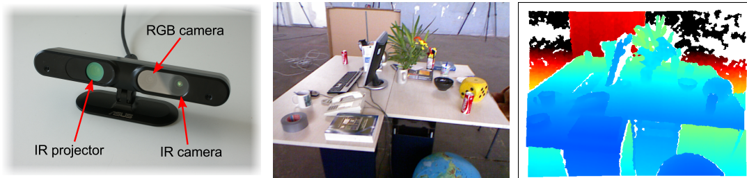
Figure 2.2.: Infrared textured light cameras provide RGB and depth images at good quality and high framerates. Left: Asus Xtion Pro Live. Center: RGB image. Right: Depth image (depth color coded).
