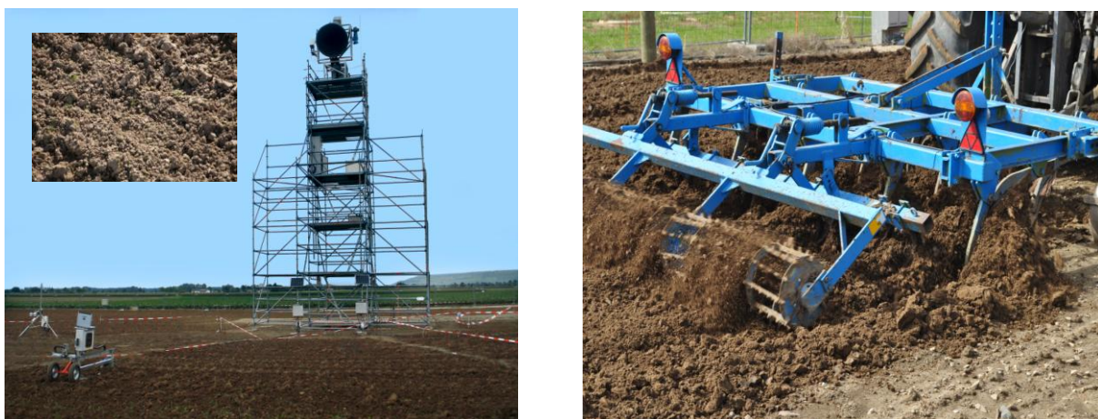
Figure III.1 L-band radiometer JÜLBARA and laser profiler over the plot (left). Mechanical field preparation (right).
