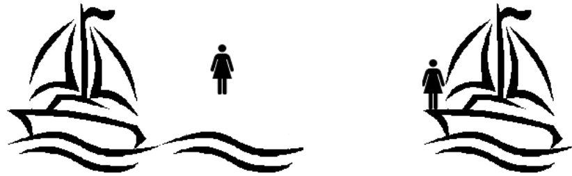
Figure 2.4.: Eulerian vs. Lagrangian point of view in fluid dynamics: The Eulerian point of view is similar to looking at the fluid while standing on the bank of the river and the Lagrangian point of view corresponds to standing in a boat, which follows the movement of the fluid.
