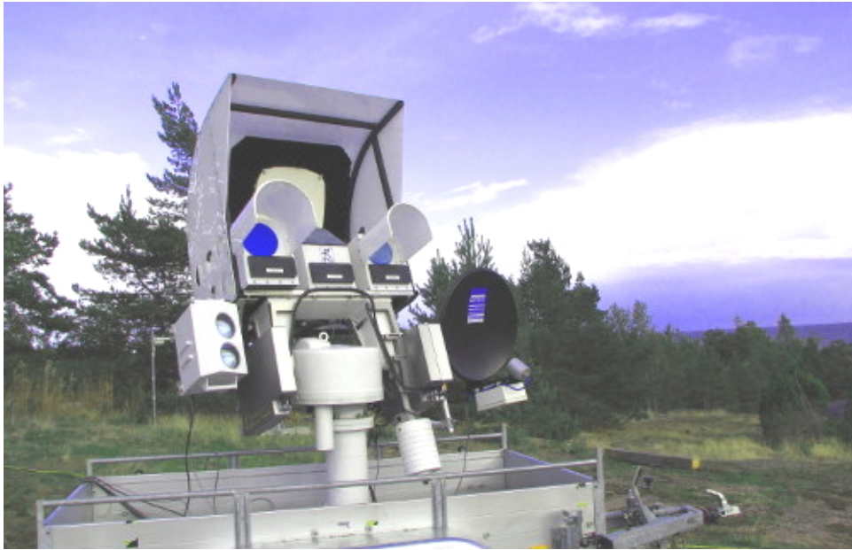
Figure 3.2.: Radiometer ADMIRARI at its standard operational configuration. Mounted on a transportable trailer. Note the ancillary instrumentation: on the left a cloud-lidar and on the right a MRR. (photo credit: P. Saavedra).
