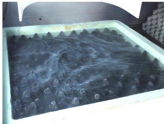
Figure 3.5.: ADMIRARI set-up for Liquid Nitrogen calibration 3.5(a), with the cold target positioned below the antenna 3.5(b). (photo credit: P. Saavedra)
