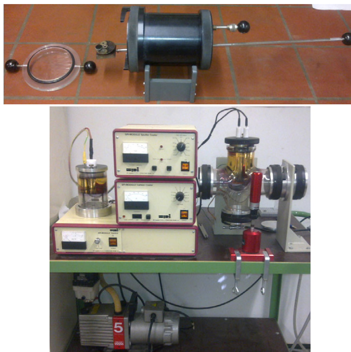
Fig. A 5.1.4.1 Transfer chamber with sample holder (top) and SPI Sputter Coater (bottom).
