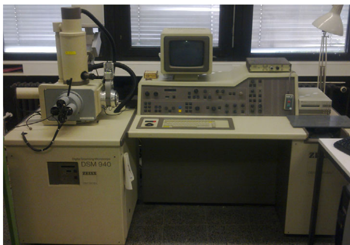
Fig. A 5.1.4.2 Scanning Electron Microscope ZEISS DSM 940. The control unit can be seen on the right side. The left modular unit consists of the turbomolecular pump (bottom) and the examination chamber with electron source and nitrogen dewar (top).
