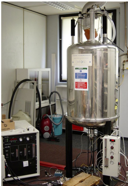
Fig. A 5.1.6.1 NMR spectrometer Varian Infinity+ with open sample holder on the bottom. The rotation control unit is shown on the left.
