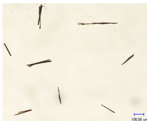
Fig. 2.9.1.5 Crystals of (SbTe 4 )[Ga 2 Cl 7 ] immersed in perfluorinated polyether.
