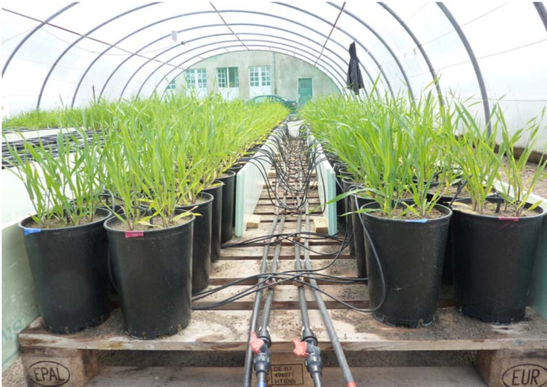
Fig. 6 Barley growth conditions of the field experiment. Plants were grown in 22 × 22 cm plastic pots containing 11.5 L of Terrasoil® in a plastic greenhouse tunnel. This allows to have natural growth condition under water-controlled conditions. Water was supplied with a computer mediated drip irrigation system to control the VWC (volumetric water content) in each pot.
