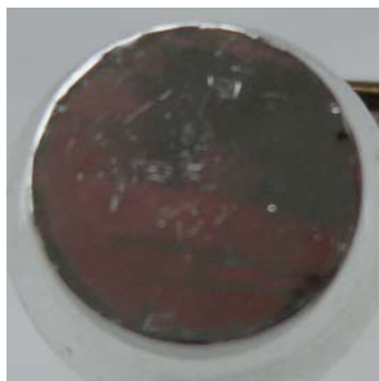
Figure 4.10: An actual photo of the Se nanoparticles on Rh(111) electrode surface.
