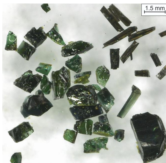
Figure 4.11 Photograph of (VO)_2P_2O_7 crystals obtained from a melt by slow cooling.
