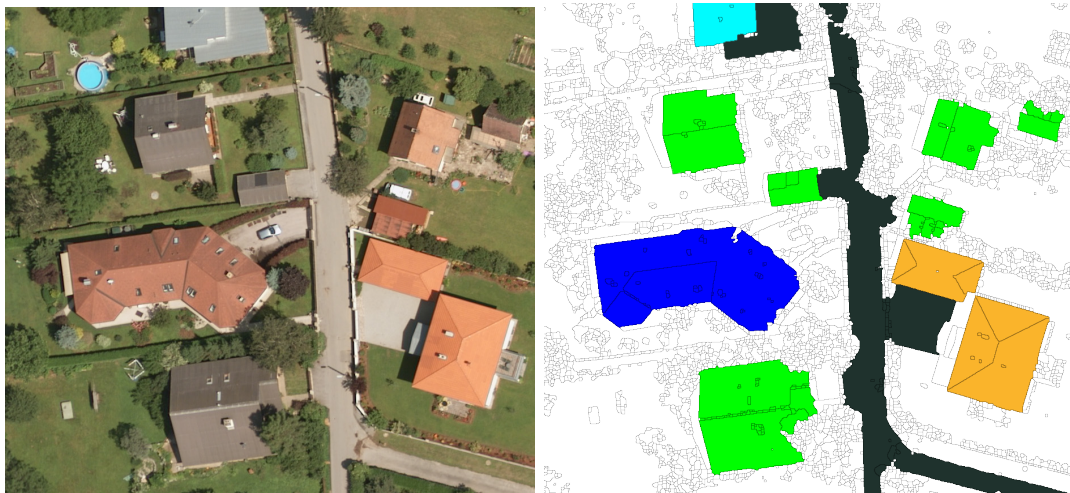
Figure 1.1: Goal of this thesis is to interpret the aerial image on the left side and get an interpretation result like shown on the right side. The colors define the different object classes. In this case there are streets [black], saddle roofs [green], hip roofs [orange], flat roofs [light blue] and other roofs [dark blue] found.
