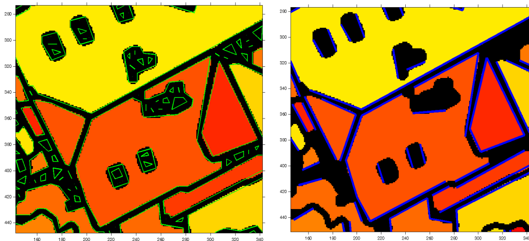
Figure 4.2: The image on the left shows the region boundaries of the extracted regions. Out of these edge-chains, the straight lines (here with a length > 25 pixel) are extracted (right image). These are stored as feature properties per region in the feature adjacency graph.
