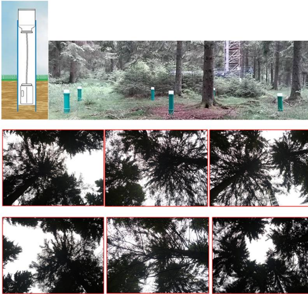
Figure A1. UMS deposition collector RS200 schematic (available at http://www.ums-muc.de ) used as funnel TF samplers with upward view, indicating the covered heterogeneity of the canopy structure.
