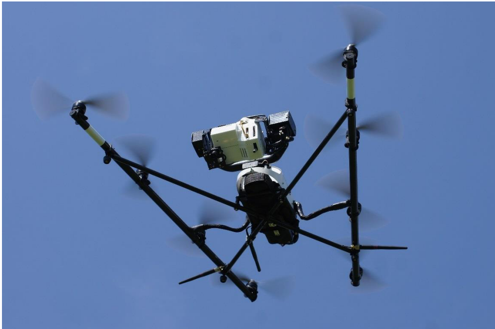
Fig. 1 Falcon-8 UAV used within the present study, during flight, equipped with the UAV spectrometer.
