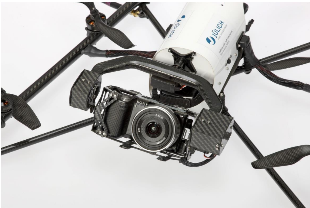
Fig. 2 Sony NEX-5n camera attached to the Falcon-8 UAV. Image provided by Ralf-Uwe Limbach.
