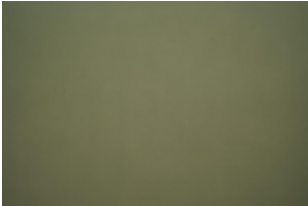
Fig. 3 RGB image averaged from >1000 different images. The image represents the vignetting pattern of the Sony NEX-5n 16 mm lens camera setup. The corners and edges appear slightly darker than the center of the image.
