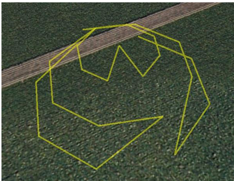
Fig. 6 exemplary path as flown by the UAV over an agricultural area to act as a goniometer. On each nook of the flight pattern, the UAV stops and points and triggers the spectrometer towards the center of the hemisphere, described by the path. Visualization captured from Google Earth.
