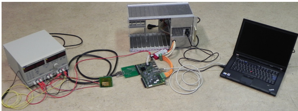
Figure 4.10: Complete Timepix SRS readout chain with single chip, external power supply, FEC and Eurocreate with power supply and computer.
