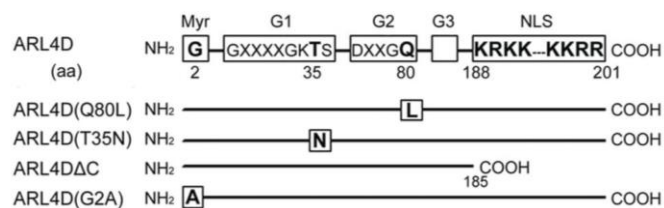
Figure 5. Schematic structure of wild type Arl4d and its mutants (Li et al., 2007).
