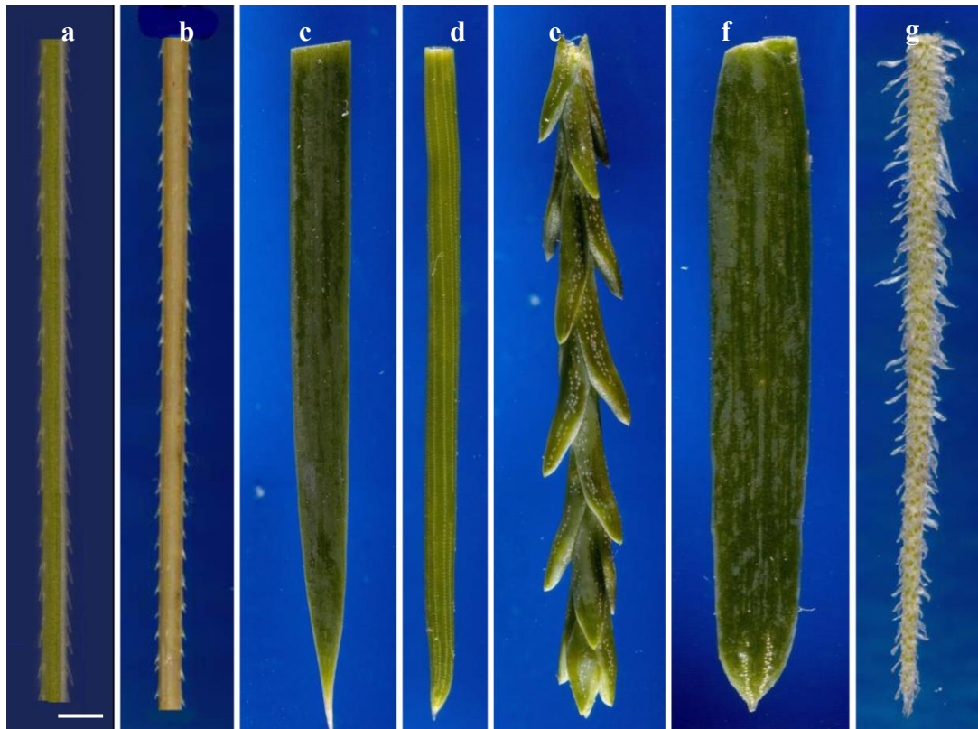
Figure 3.3: (a–g) Optical photo of awns, needles and leaves used in the fog-collection experiment; scale bar 1 mm. (a) A fresh and (b) a DH awn of Hordeum , (c–f) needles/leaves of Abies , Pinus , Sequoiadendron and Sequoia , respectively and (g) a leaf (needle like structure) of Tillandsia . Published in Azad et al 2015a.
