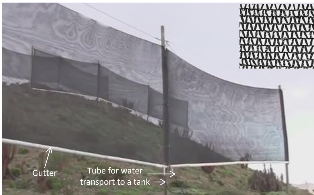
Figure 1.4: Large fog collectors (LFCs) made of double layer polyolefin mesh located in the Atacama, Chile. (reproduced from: https://www.youtube.com/watch?v=2x2_8RbC2i0 ; accessed on 22.07.2015). The inset shows the fiber network of a single layer polyolefin mesh (modified after Klemm et al 2012; Copyright Royal Swedish Academy of Sciences 2012)
