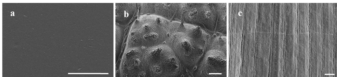
Figure 5.1: Scanning electron micrographs of (a) a smooth surface of a glass replica, scale bar 200 \mu\text{m} ; (b) a papillate surface with random channels and hairs inside the channels of Gunnera leaf replica, scale bar 300 \mu\text{m} and (c) a microgrooved surface of Dendrocalamus leaf replica, scale bar 300 \mu\text{m} .
