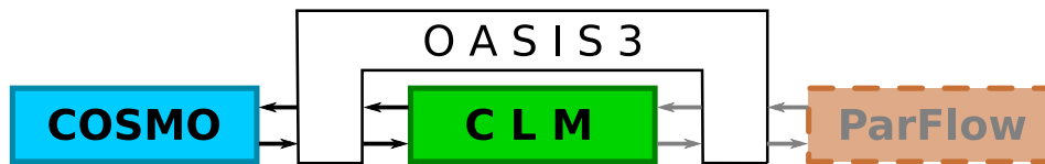
Figure 2.1.: TerrSysMP, a model platform consisting of the COSMO model (version 4.21), CLM (version 3.5) and ParFlow, externally coupled with OASIS3.
