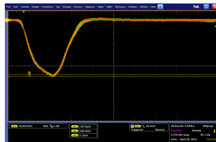
(c) PMT orthogonally orientated to magnetic field (figure 4.13b). Helmholtz coils turned on and without shielding.
