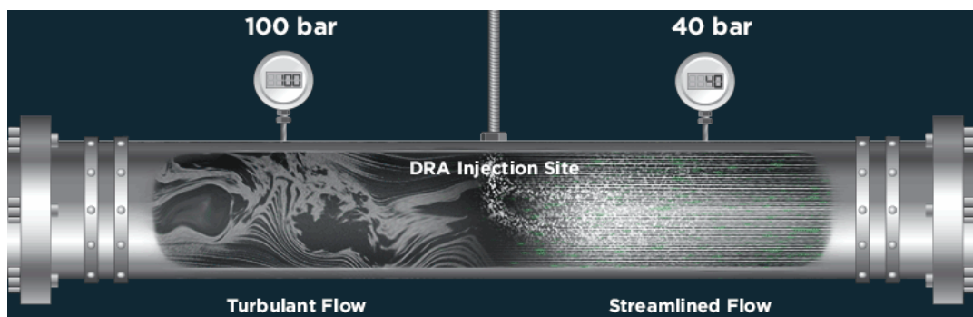
Figure 0.2.: Illustration of turbulent drag reduction for oil transport in a pipeline. The drag reducing agent (DRA) is added at the channel's center and changes the turbulent oil flow into a laminar flow. The figure is taken from an advertisement for the TURBOFLO DRA by Flowchem [62].
