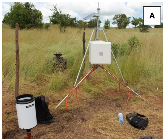
Fig. 4-5 Soil water station. Part A shows an external view of the station and part B shows one of the two profiles of the station. For each profile 3 FRD probes and 3 pF-meters are installed per soil horizon (A-horizon and B 1 -horizon, see Fig. 4-10 for profile description).
