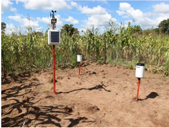
Fig. 4-1 Climate station (Yabogane site) recording rainfall [mm], air temperature [ ^{\circ}\text{C} ], relative humidity [%], wind speed [ \text{m s}^{-1} ] & direction [ ^{\circ} ], solar radiation (incoming short wave) [ \text{W/ m}^2 ], storage interval: 5 min.
