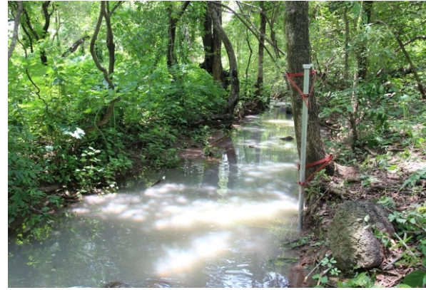
Fig. 4-2 Gauging station (Dano-Paré site). Recording water level [mm], storage interval: 10 min.
