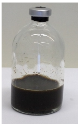
Figure 8: Batch incubation system. 20 g biogas sludge incubated anaerobically in a 120 ml serum bottle.
