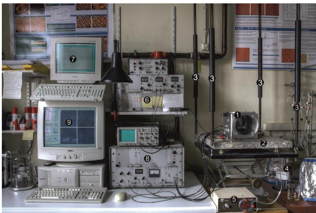
Figure 3.2: Picture of the EC-STM system: 1) aluminium chamber for the STM; 2) heavy granite plate; 3) steel springs connected with the ceiling; 4) electrolyte supply and gas purification system; 5) hose pump; 6) bipotentiostat; 7) computer for displaying the cyclic voltammograms; 8) STM control unit; 9) computer for controlling the STM unit and displaying STM images.
