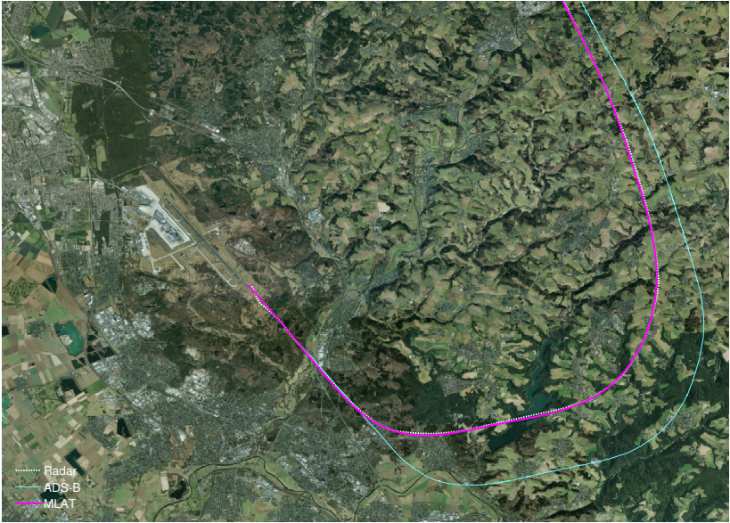
Figure 4.20: Example 1. Aircraft departing at CGN projected over satellite image. (Map Data: ©GeoBasis-DE/BKG 2016).
