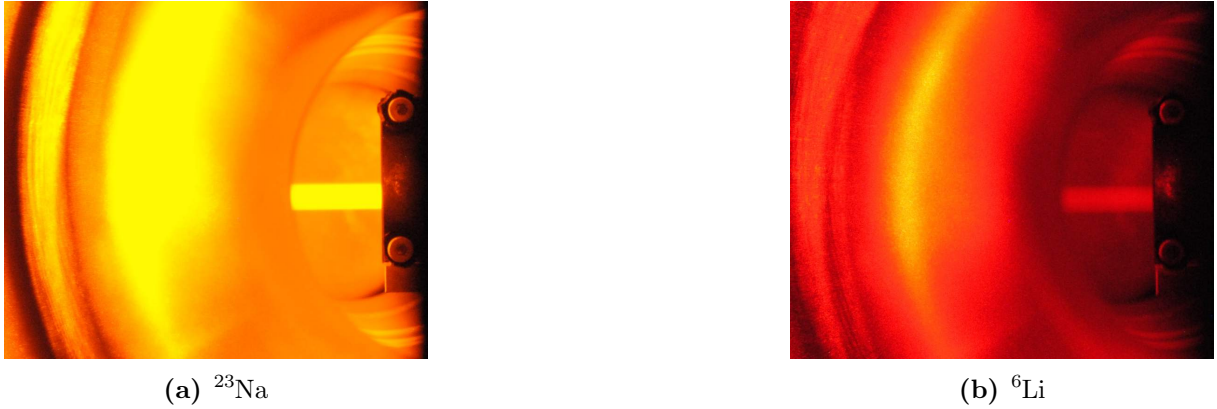
Figure 4.1: Fluorescence of the collimated atomic beam from the incident Zeeman slower beam for ^{23}\text{Na} (Fig. 4.1a) and ^6\text{Li} (Fig. 4.1b). The pictures are taken from the sapphire window in the oven chamber. The exposure time for ^6\text{Li} is approximately 10 times larger than that of ^{23}\text{Na} .
