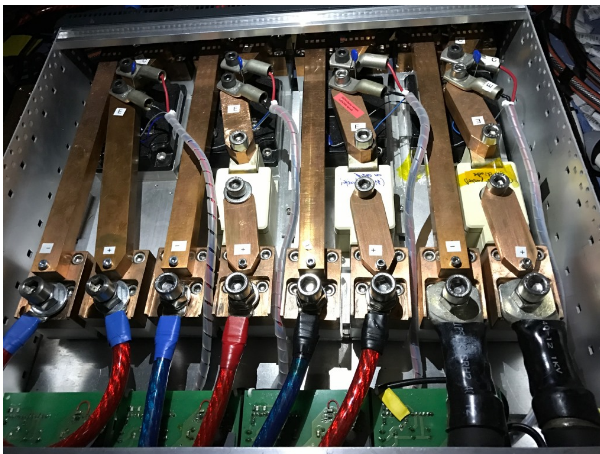
Figure B.10: IGBT Box 1 has 4 channels (each with a single sub-channel). The IGBT modules are the black structures towards the back of the image. The white components in the center are the 600 A diodes. The PCBs visible at the bottom of the image are the IGBT driver boards. The wires at the bottom go directly to the coils and connections at the back of the box go to the power supplies. The plate at the bottom is water cooled.
