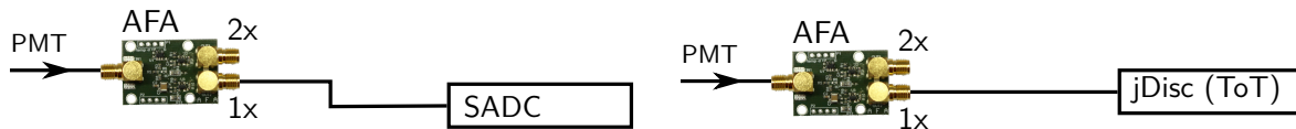
(a) Direct connection to the SADC input with AfA in front (necessary since the SADC introduces a DC offset on the input). (b) Direct connection to the jDisc module with AfA in front to be able to disentangle AfA effects.
