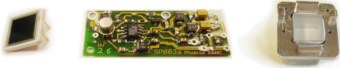
Figure 7.15.: The components used to build up the real-time and in-situ detector used in the collector chamber of the BONIS facility. From left to right: Hamamatsu's S8664-1010 APD with polished surface, the charge sensitive preamplifier SP883a [Honisc15] and the LYSO:Ce crystal wrapped in PTFE tape and inserted in its Al case. All components are roughly to scale.
