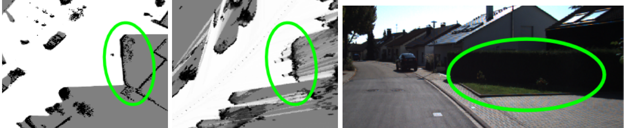
Figure 5.39: Detected error in the reference map. The green circles show that a small bush is missing in the reference data (left), but is clearly mapped using our new mapping approach (middle).
