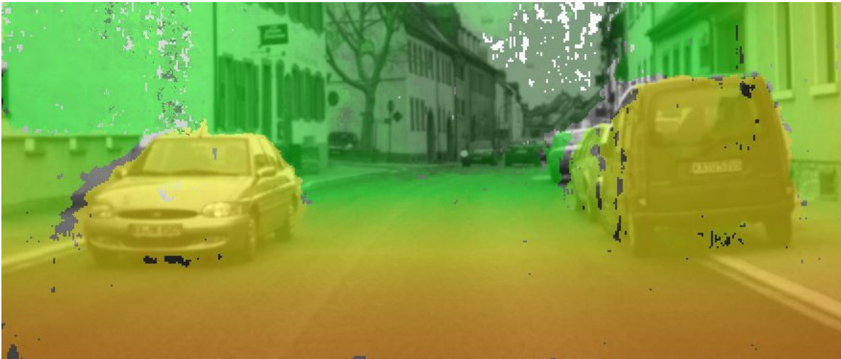
Figure 2.4: Dense disparity image via semi-global matching (SGM). The color encodes the distance. Red stands for near, green for far away obstacles. For nearly each image point a disparity information is computed (excluding stereo shadow). Equations (2.4)-(2.6) are used to estimate the 3D scene points.
