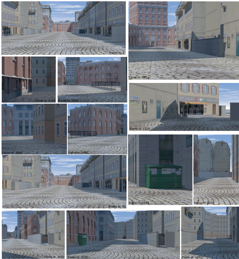
Figure 5.1: Example images of the self generated 3D city model. The open source library POV-Ray is used to create the virtual environment. A realistic engine model is applied to define the GT vehicle path. Each single 3D point of the city model is known which allows us to generate the GT occupancy grid map \mathcal{M}_{GT} . We also utilized the 3D city model to render artificial stereo image sequences which are the basis for our mapping approach (see Fig. 5.3).
