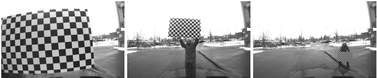
Figure 2.2: Example images of a planar calibration rig. These images are used to estimate intrinsic parameters for mono cameras (left image) as well as to calibrate stereo camera system (middle and right image).
