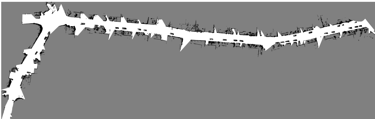
(b) Reference occupancy grid map for sequence 0064, 450 \times 160 m
