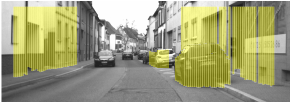
(a) The static Stixel set \mathcal{S}_t limited up to 40 m.
