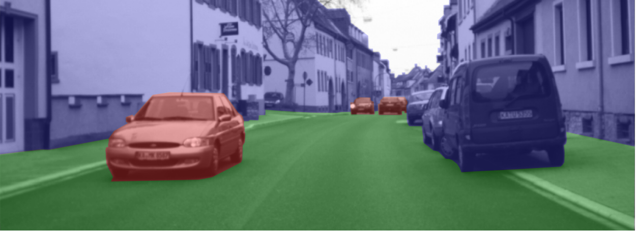
Figure 1.1: The classification of an urban traffic scenario into dynamic objects (red), static information (blue) and free space (green) which also includes the sidewalk. The detection of these three types is mandatory for advanced driver assistance systems and autonomous driving applications [Ziegler et al., 2014].
