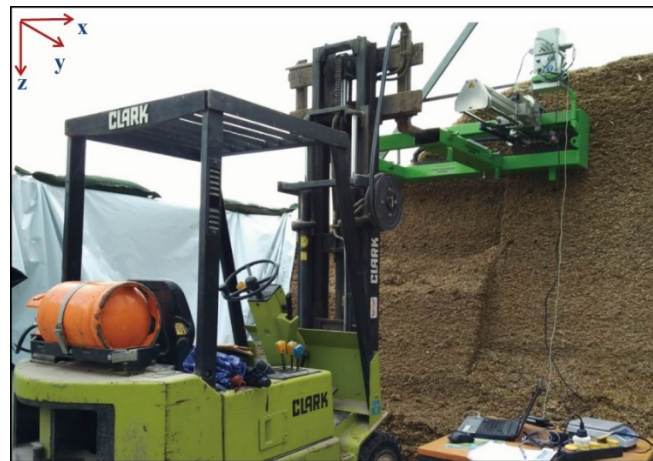
Figure 20 Using a forklift to position the frame prior to penetrating the face of the bunker silo at different heights
