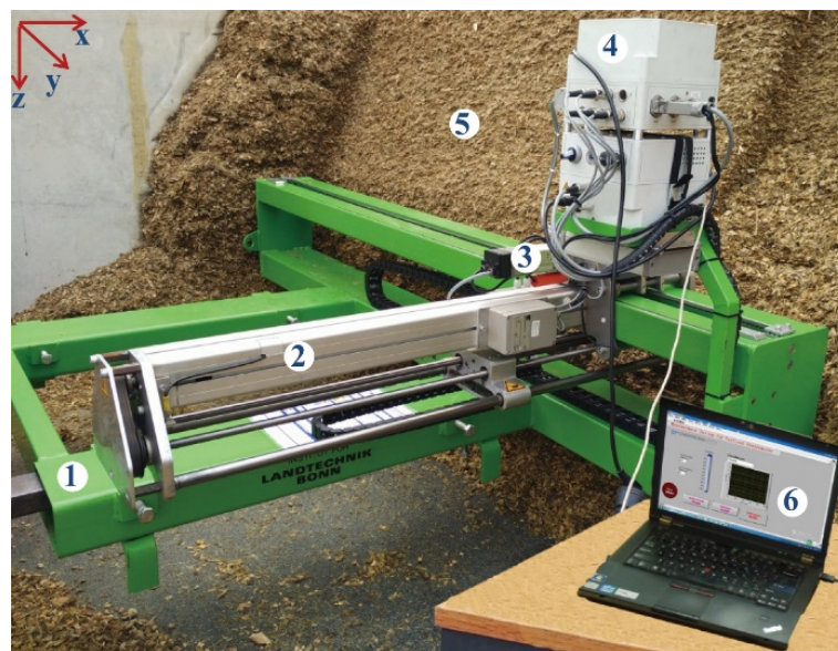
Figure 18 A photo of the penetrometer-based mapping system: 1) frame, 2) penetrometer, 3) motor for y-axis translation, 4) relay-box, 5) maize silo, and 6) the interface of the measurement system.
