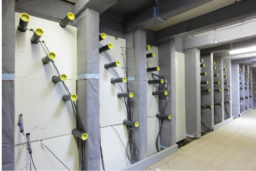
Fig. 2. 2 Interior view of the minirhizotron facility. The rhizotubes were installed perpendicular to the wall profile.
