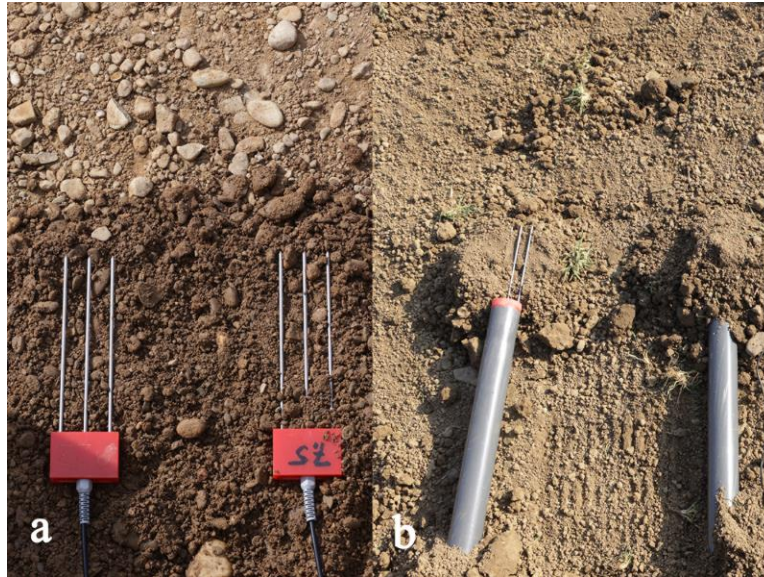
Fig. 2. 5 Time-domain reflectometry (TDR) sensors in the (a) upper and (b) lower facilities. The bases of the TDR sensors were refitted to a round shape attached to a plastic pipe for inserting into the bored holes in the lower facility.
