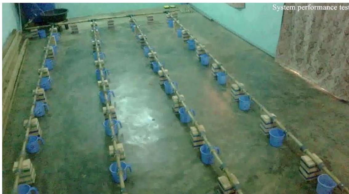
Figure 2.5 Test of emitter flow uniformity in the bamboo-drip system
