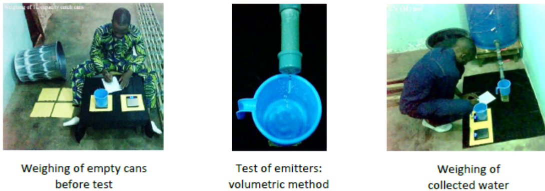
Figure 2.3 Test of emitter flow variation caused by emitter precision
