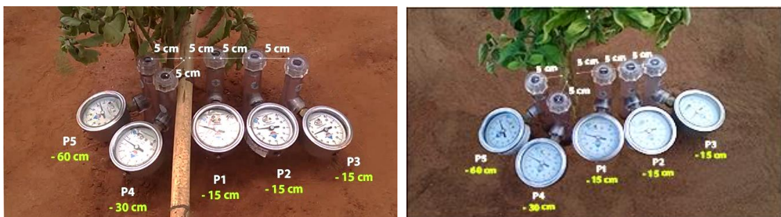
Figure 4.2 Tensiometers in drip (left) and watering-can (right) plots
