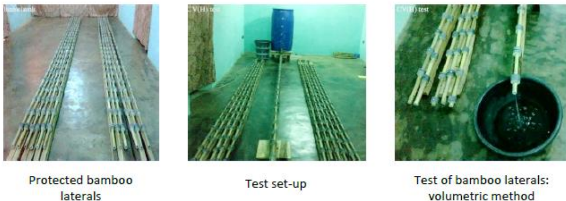
Figure 2.2 Test of emitter flow variation caused by bamboo material
