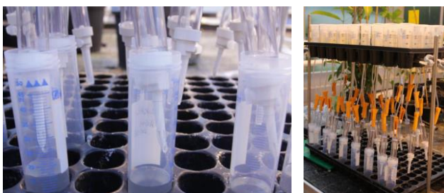
Fig. 6 Percolation tubes to analyze P mobilization from struvite after flushing the soil with citrate. The orange syringes regulate the leachate that is collected in the tubes shown in the right picture.
