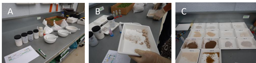
Fig. 7 Overview of the fertilizer blending process in the organic substrate: a) Recovered nutrients as delivered; b); blend preparation before grinding; c) overview of the different blends before mixing with the substrate
