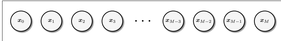
(a) EKF: runs online, but contains only the current state variable and does not iterate.
